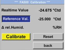
Here, a one-point calibration can be performed
