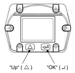
The operation of the FA 500 is done by the two capacitive key buttons Up ( $\triangle$ ) and Enter ( $\downarrow$ )
